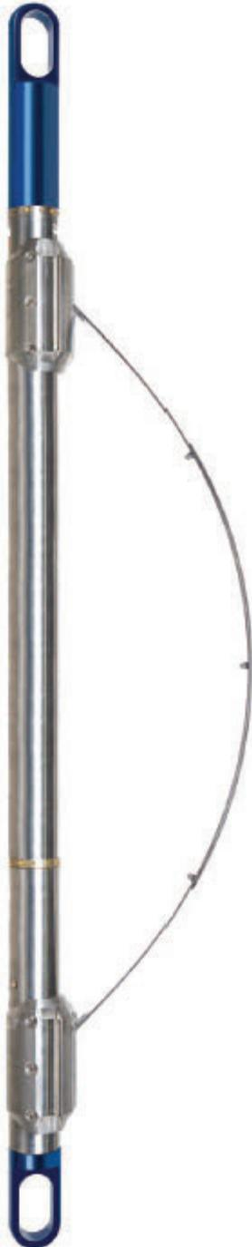
The Compensated Neutron (CNL) tool measures the hydrogen content of the formation surrounding the wellbore. The hydrogen content is related to porosity, and can be used for gas detection in combination with other tools in both open and cased hole applications.
